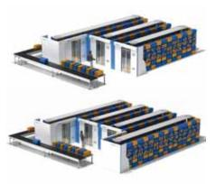
Triple stations or quadruple stations are recommended for applications with a wide range of items that require frequent access – the layout is usually L-shaped.
